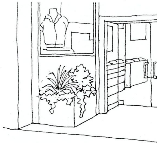
Landscape planter bulkhead
